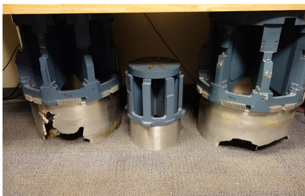
Figure 1: Catastrophic failure due to an electrodynamic shaker being driven at a resonance in which the armature bends, leading to excessive stresses in the cylindrical part that is shown.
