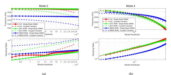
Figure 2: Dynamic responses with multi-mode excitation where Mode 4 has 10x the peak excitation amplitude of Mode 2. (a) Mode 2, (b) Mode 4. The results are compared to single-mode QSMA predictions for reference.
