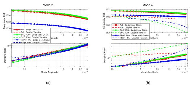
Figure 2: Dynamic responses with multi-mode excitation where Mode 2 has 10x the peak excitation amplitude of Mode 4. (a) Mode 2, (b) Mode 4. The results are compared to single-mode QSMA predictions for reference.
