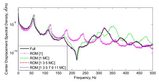
Figure 8. Autospectrum of the midpoint transverse displacement to a random force input with a standard deviation of  $\sigma = 0.1$  lbf.
