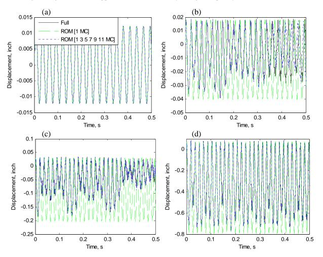
Figure 7. Response of contacting DOF due to a half-sine pulse in the shape of the first linear mode with system energy of (a)  $E = 1.8 \cdot 10^{-4}$  in-lbf, (b)  $E = 2.0 \cdot 10^{-3}$  in-lbf, (c)  $E = 5.0 \cdot 10^{-2}$  in-lbf, and (d) E = 0.76 in-lbf. (Solid black) full order model, (dashed green) ROM with modes [1 MC], and (short dashed blue) ROM with modes [1 3 5 7 9 11 MC].
