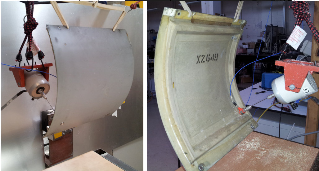
Figure 1. Photograph of the Lynx helicopter (top) and front (bottom-left) and back (bottom-right) views of the panel that was studied, suspended by bungee cords for a free-free test.
