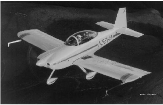
he RV-8A is an all metal, tandem, low wing, low aspect ratio monoplane like its predecessor, the RV-4. Both are creations of Van's Aircraft in North Plains, Oregon. However, the RV-8A is a distinct new design with substantially different features. It is intended to be a high performance sport plane with a mix of capabilities ranging from basic positive G. aerobatics with nimble handling qualities to limited cross country travel.
