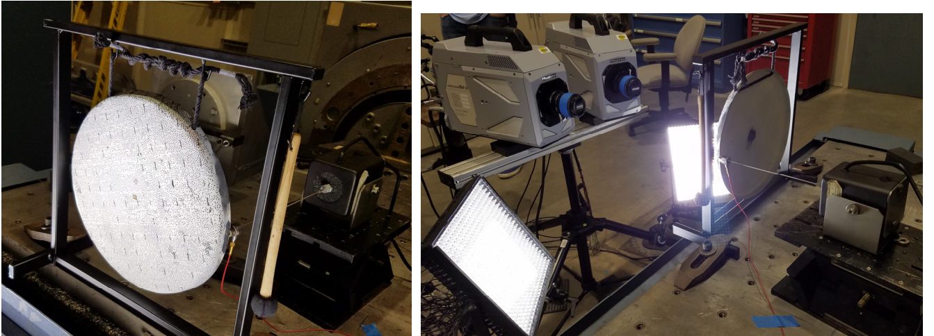
Figure 1. Photographs of setups used for DIC tests for system identification. (a) Front view of gong. (b) Photograph showing shaker setup, lighting and DIC system. Two LDVs were also used, which are part of the hardware seen behind the leftmost DIC camera.
