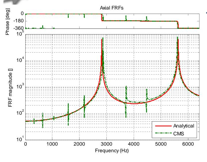
The CMS method predicts the axial FRF very accurately when the Modal Constraint for Fixture and Subsystem (MCFS) is used.
