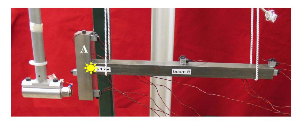
• Careful tests used to estimate the modal parameters of the C system at a number of points on fixture A.
