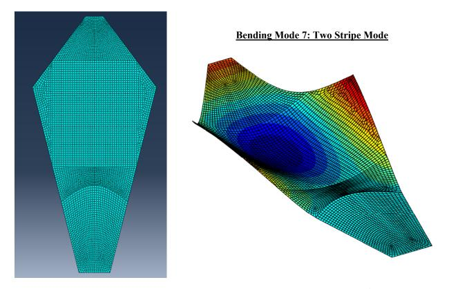
Figure 4. (left) Finite element model used to model the cantilevered flat plate (right) 7<sup>th</sup> bending mode.
