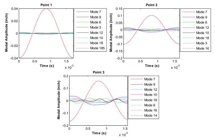
Figure 7. Time histories of the integrated response of the full order model for the points shown with black squares in Fig. 6 using the ICE (1, 3, 6, 7, 9, 10, 12) CD (10, 3, 1, 2, 1, 1, 1) ROM. The first 8 most dominant modal displacements are shown over one integration period.
