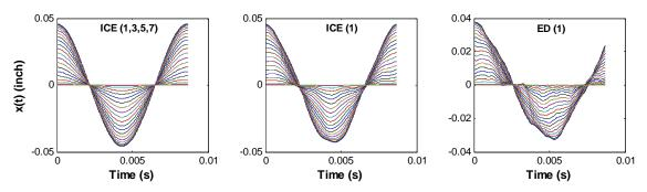
Figure 3. Time histories found after integrating the full FEA model subject to the initial conditions prescribed by each of the ROMs for the points near 115 Hz in the FEP in Fig. 2.
