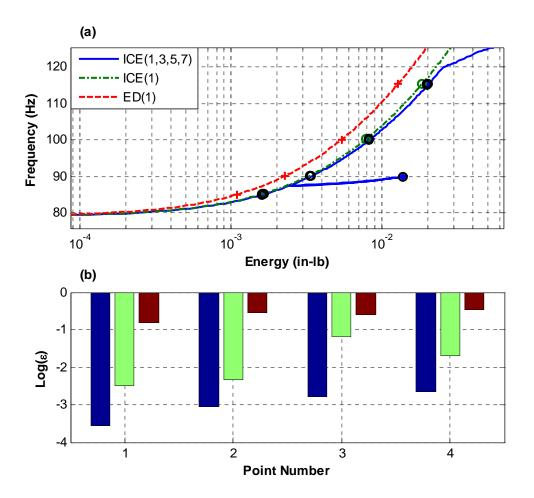
Figure 2. (a) Frequency-energy plot showing the first NNM of various ROMs, and (black circles) represent converged NNMs with the full FE model. (b) Base 10 logarithm of the shooting tolerance,  $\varepsilon$ , in Eq. (10).
