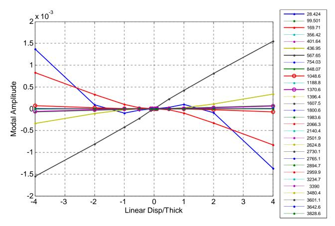
Figure 5. Force-displacement analysis of the plate when a force in the shape of Mode 7 is applied to the nonlinear finite element model. The colored lines represent the modal amplitudes of the statically coupled modes, whose linear natural frequencies are in the legend.
