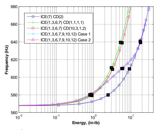
Figure 6. Estimate of 7<sup>th</sup> NNM computed from various ROMs of the cantilevered plate. In the last two lines of the legend, Case 1 corresponds to CD(10,3,1,2,1,1,1) while Case 2 used forces half as large with CD(5,1.5,0.5,1,0.5,0.5,1,0.5,0.5,0.5).
