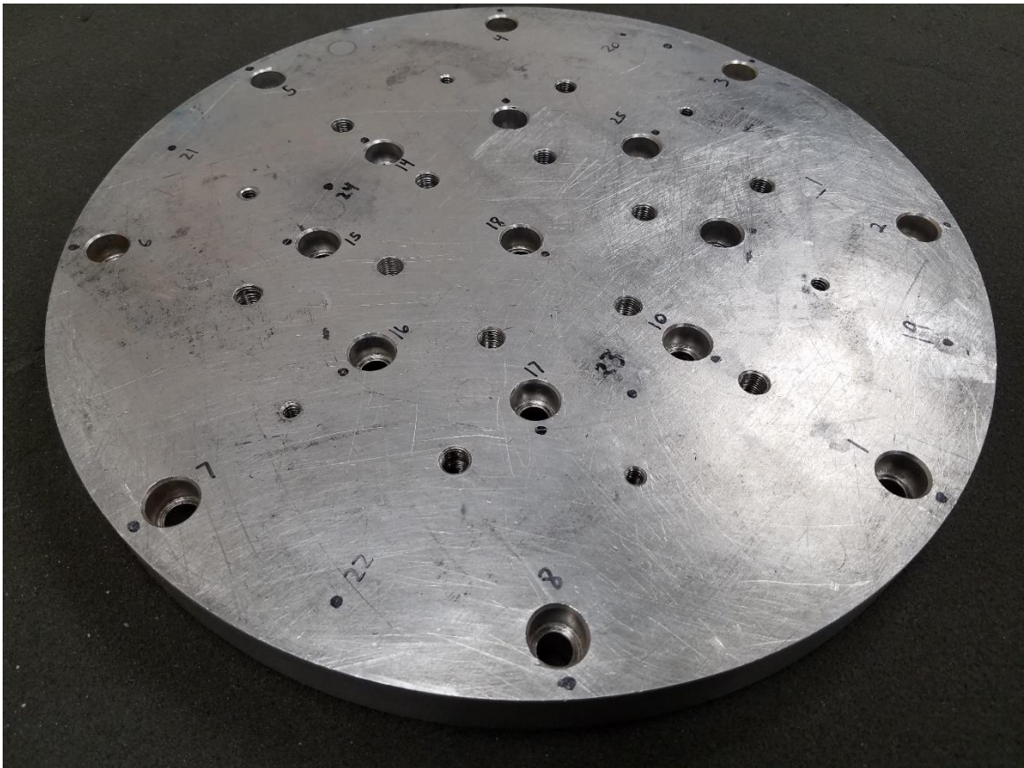
Figure 2: The Transmission Simulator, an aluminum adapter plate
