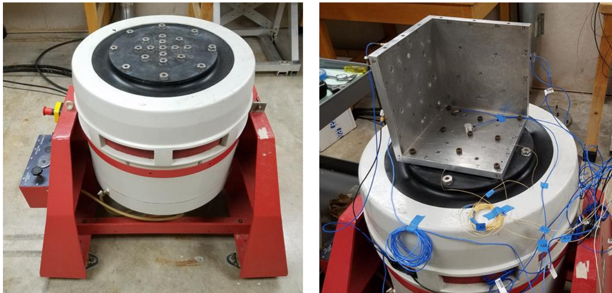
Figure 18: (Left) The shaker system used to evaluate the proposed substructuring approach, and (Right) The Experimental Subsystem; the TS mounted on the shaker.
