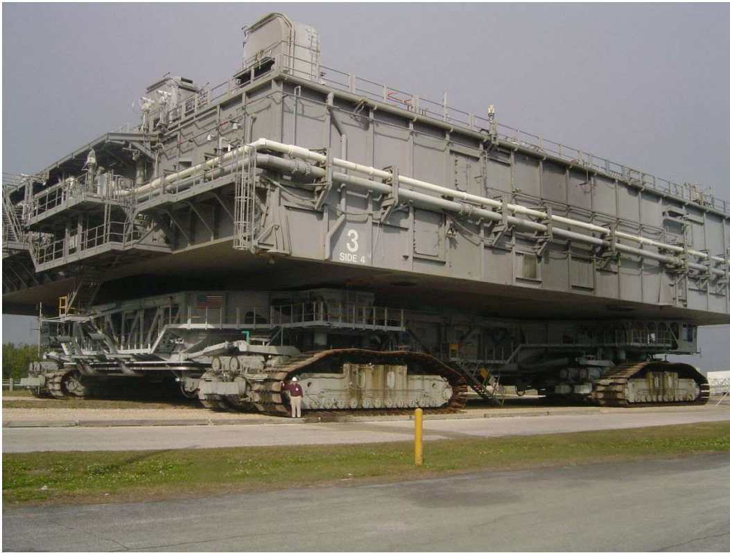
Figure A5: Crawler-Transporter (CT) Moving a Space Shuttle Mobile Launch Platform (MLP)
