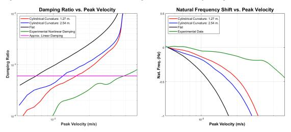
Figure 2: Effective Natural Frequency and Damping of flat and curved interfaces compared to experimental data.
