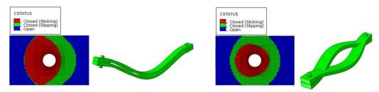
Figure 1: Joint interface slip contours and mode shapes for mode 2 (left) and mode 6 (right).
