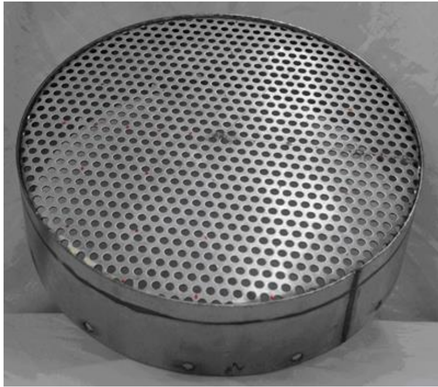
Figure 2: Perforated plate welded into supporting cylinder
