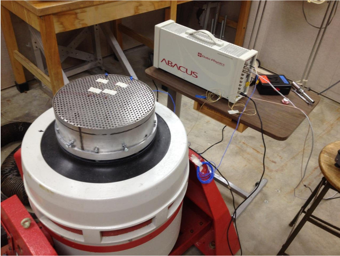
Figure 22: Experimental Setup with Ling Dynamics V830-335 SPA10K (RM) modal shaker and ABACUS data acquisition hardware
