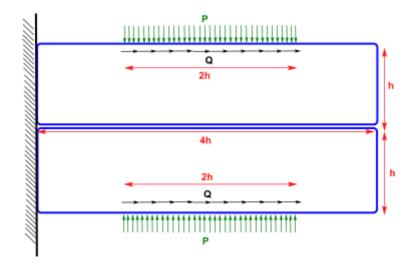
Figure 1. Beam structure with a clamping load representing a bolted joint and a shear load which exercises the joint.
