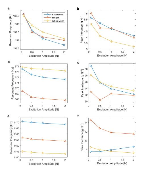
**Fig. 1** Comparison between experiment and the modeling approaches of (a,c,e) the resonant frequency and (b,d,f) peak intertances in the (a,b) first, (c,d) second, and (e,f) third bending modes of the Brake-Reuss beam.
